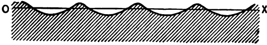
FIG. 134.— Showing that a surface disturbed by ripples is larger than a level surface.
